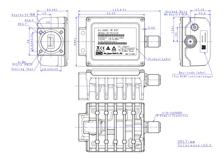
Caution: <u>DO NOT</u> remove the sealing tape on the waveguide. If the sealing tape is removed, it may lose the performance of waterproof.
